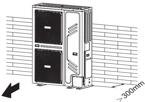
In case of strong wind and the wind direction can be foreseen, refer to the figures below for installation of the unit (any one is OK):
