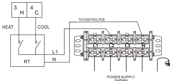
There are three methods for connecting the thermostat cable (as described in the picture above) and it depends on the application.
