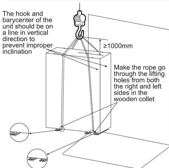
The position of barycenter for different unit can be seen in the picture below. (unit:mm)
