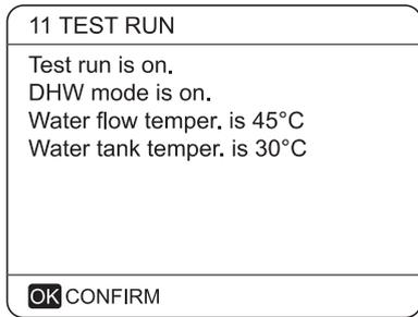
During DHW MODE test running, the default target temperature of the domestic water is 55°C. The TBH (tank boost heater) will turn on after the compressor runs for 10min. The TBH will turn off 3 minutes later, the heat pump will operate until the water temperature increase to a certain value or the next command is received.
