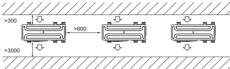
3) Parallel connect the front with rear sides
